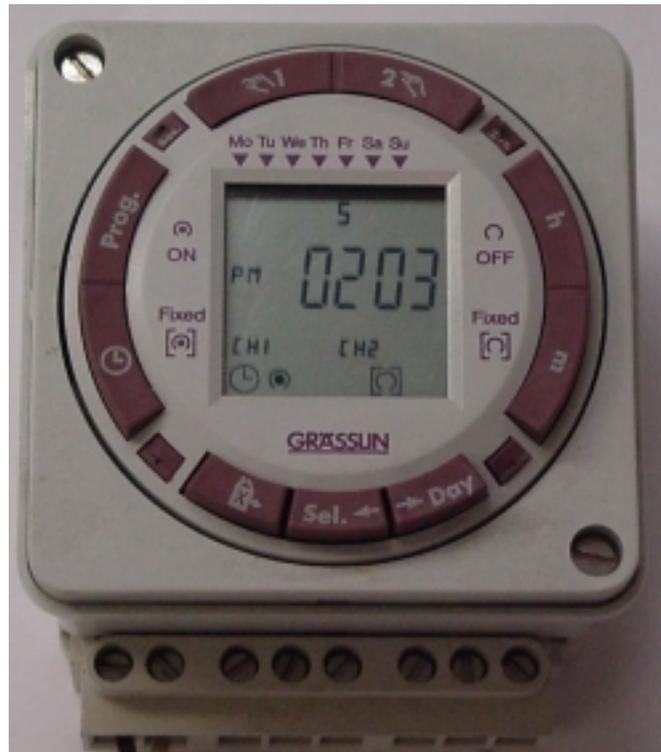
ACS's Lighting Control (LC) Panel uses a two-channel programmable time switch shown above.
